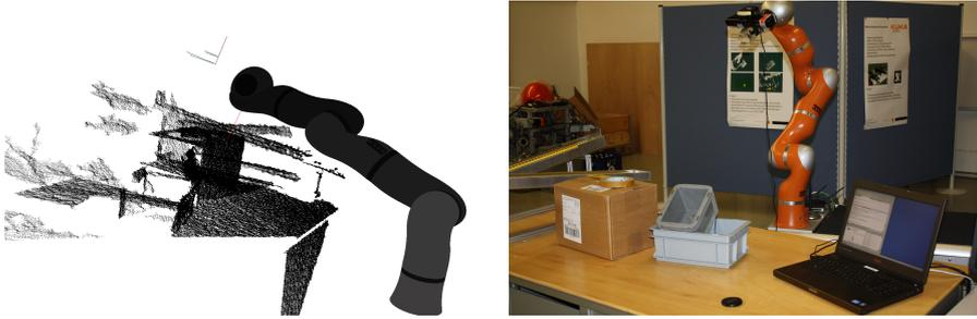
Figure 7.10: A typical point cloud recorded by the Kinect and the polygonal model of the LWR. The red line denotes the minimum distance between the LWR and the point cloud (left). The complete setup of our application: The KUKA Omnirob with a head mounted Kinect in front of a workspace (right).
